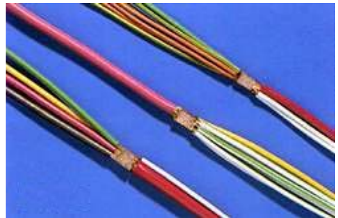
Fig. 1 The ultrasonically welded copper wires
