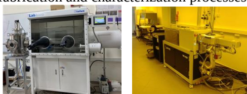
Figure 1. Images of (a) glove box and (b) ALD systems
