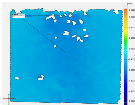
Figure 9 Map of the displacements of primary load reaching the value of 125 kPa
