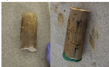
Figure 2-2 MICP treated samples after being removed from the tube, discoloration visible at the top showing a change in colour at the surface. Left B4 treated sample after 21 days. Right Deionised water treated sample after 21 days
