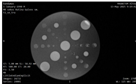
Fig. 14. Low-contrast object detectability evaluation on Siemens Magnetom Altea (1.5T) system with T_1 -weighted images
