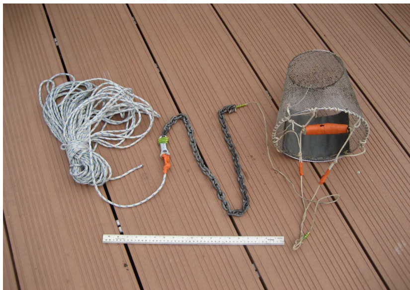
Figure 2. Basket dredge used to retrieve Asian clams during 2011 and 2012, scale is 50 cm.
