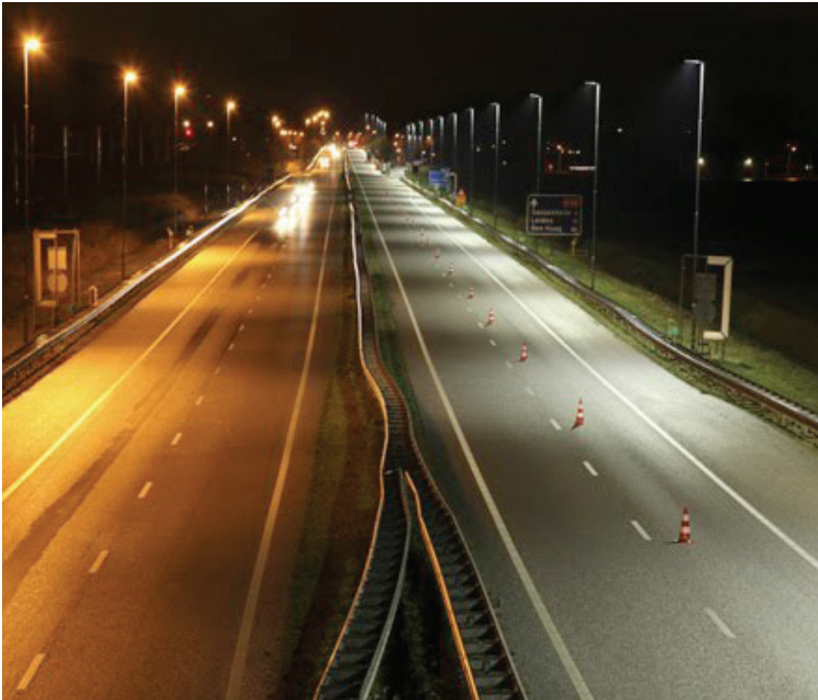
The difference in colour perception between LPS (left) and LED (right)
