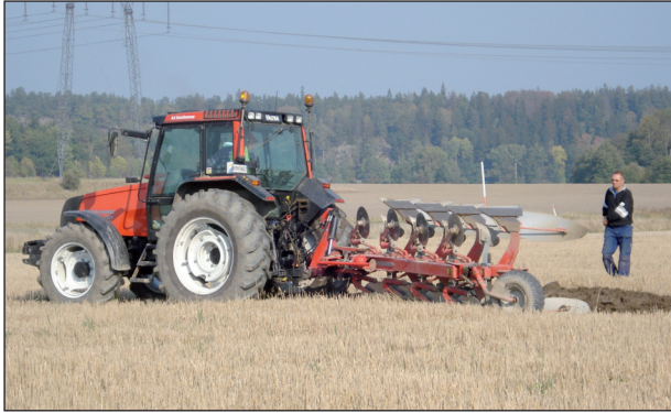
Figure 9.11. A reversible plough for conventional ploughing to the depth of 23 cm. Photo: B. Ulén.
