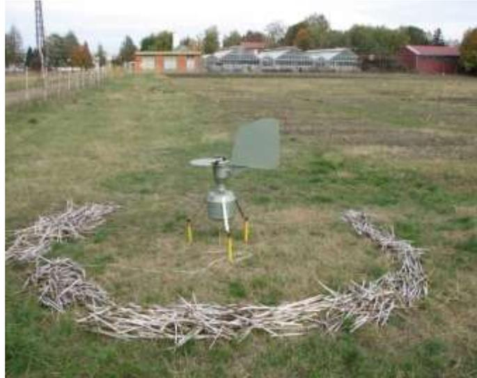
Fig.1.Burkard spores catcher
