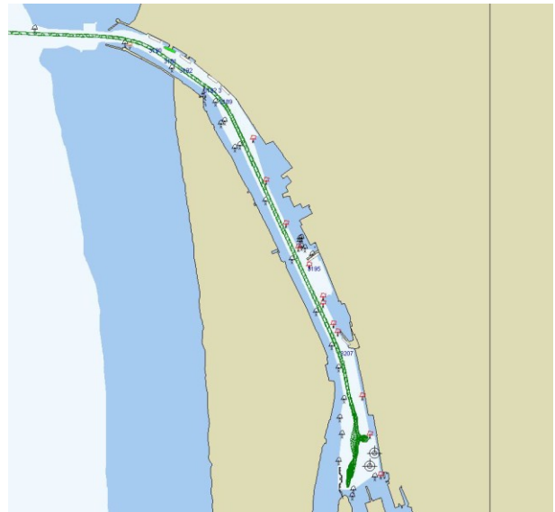
Fig. 2. LNG tanker sailing trajectory from entrance to the port until the mooring place
