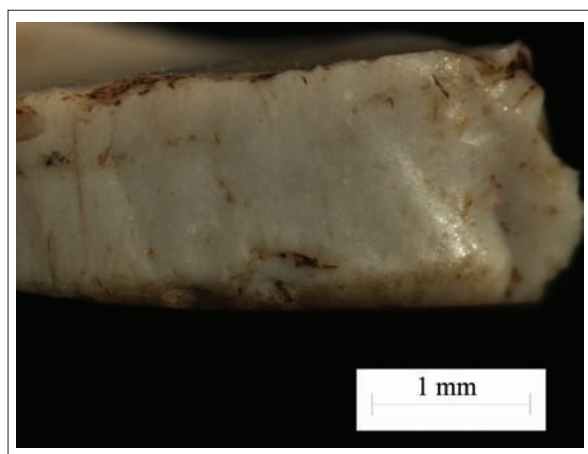
Fig. 13. Use-wear retouch on the pin of burin. 16x (photograph by G. Slah).
