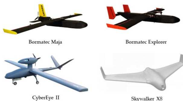
Fig. 2. Fixed wing vehicles for RPAS [5].
