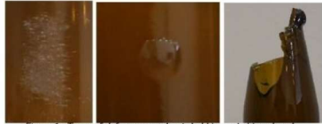
Figure 1: Types of defects: scratch, air bubble, and chipped neck
