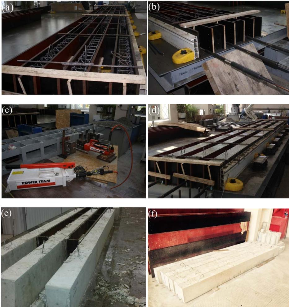
**Fig. 3.5.** Preparatory works prior experimental tests: mounting of the formworks and reinforcement cages (a); installation of prestressing reinforcement (b); mounting of hydraulic jack (c); casting of concrete (d); visual quality inspection due to honeycombing (e); cut-off prestressing reinforcement, lifting and storage (f)
