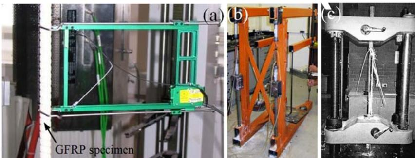
**Fig. 1.7.** Experimental testing equipment: tension – tension test of glass composite bar (Atutis *et al.* 2015) (a); creep test of basalt composite bar (Banibayat 2015) (b); tensile test setup for aramid fiber reinforced polymer bar (Zou 2003) (c)
