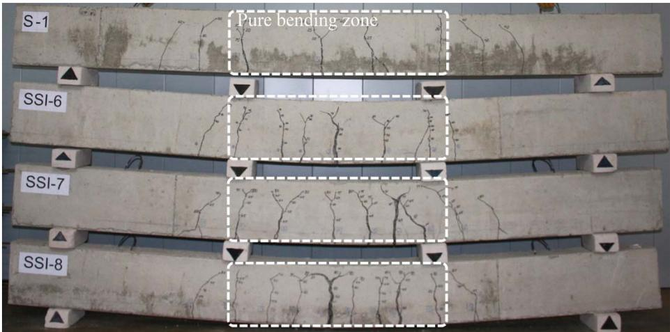
**Fig. 3.12.** Cracking pattern of Series 2 versus control beam
