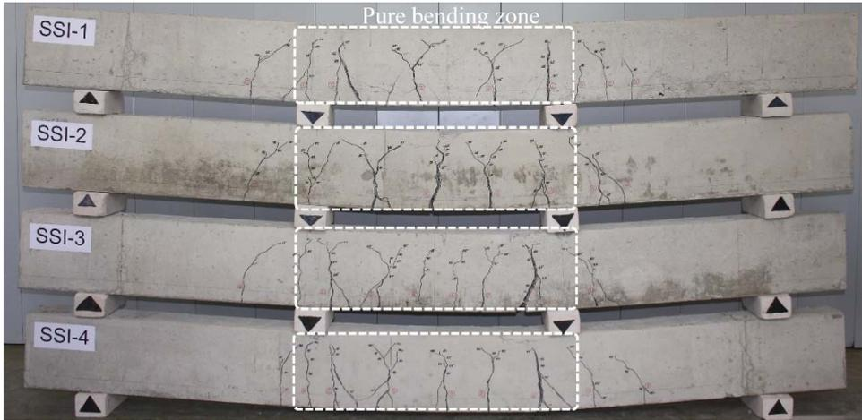
**Fig. 3.9.** Cracking pattern of beam Series 1
