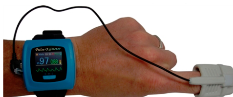
Figure 1. The CMS50FW wearable oxygen saturation (SpO 2 ) and pulse rate device with wireless communication for real-time vital-sign monitoring.
