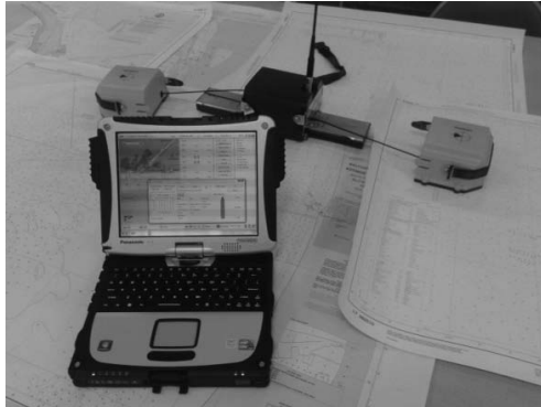
Fig. 1. Very high accuracy navigation system, „E-Sea Fix“, which has accuracy of ship’s position in RTK mode – +/- 2–5 cm
