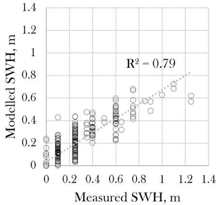
Figure 11. The comparison of observed and modelled SWH in the Ventè validation station.
