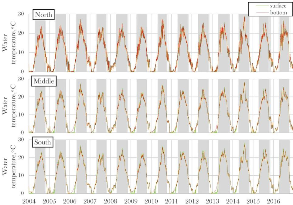
*Figure 35.* Comparison of water temperature along the three Curonian Lagoon stations: in the north (55.573414°N; 21.157354°E; depth 2.38m), in the middle (55.314449°N; 21.123343°E, depth 3.33m) and in the south (55.030495 °N; 20.917892°E, depth 4.17m). Grey area indicates the period when the new formula for settling velocity was activated.
