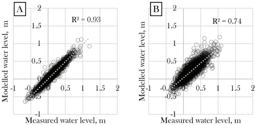
Figure 10. The scatterplots of the observed and modelled parameter values. (A) Water level in the Klaipėda station, and (B) water level in the Nida station.
