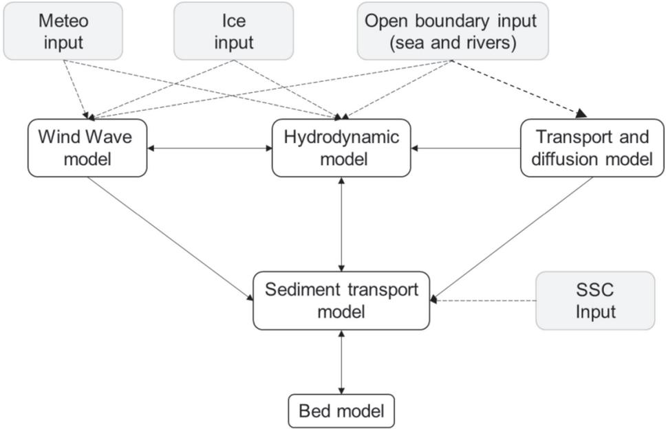
Figure 2. The SHYFEM model structure for this study.
