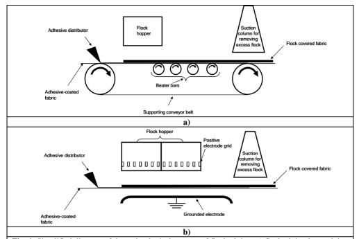
**Fig. 1.** Simplified diagram of the technological process of flock gluing: a) flock gluing by applying the vibrational method; b) flock gluing by applying the electrostatic method
