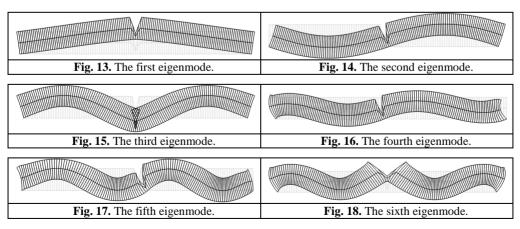
The obtained results of experimental investigation indicate that the character of some of the eigenmodes of vibrations under the influence of defect undergoes essential changes: for
