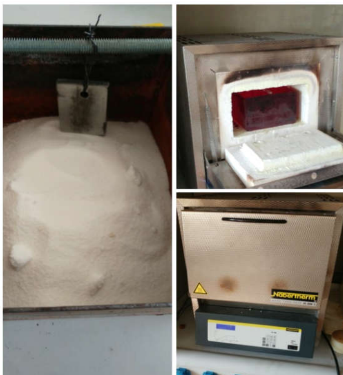
Fig. 11. Nitriding of samples in Potassium Nitrate Salt
