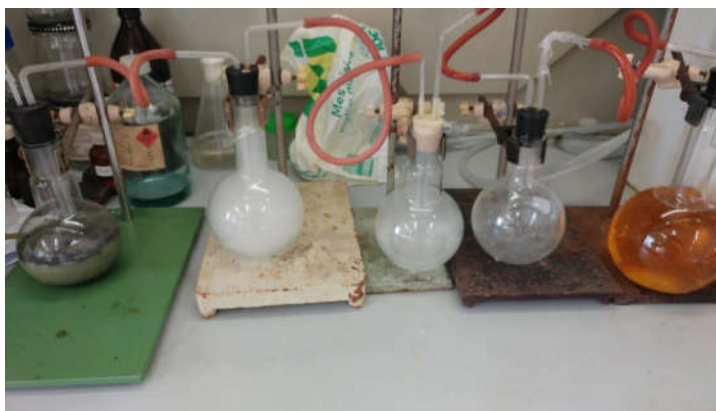
Fig. 14. Basic setup (NaCl in this case) for measuring the corrosion rate of the metal samples
