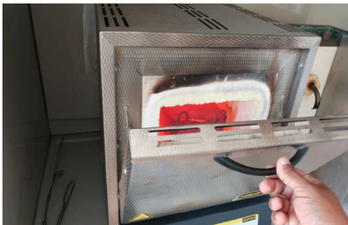
Fig. 9. Heated in a thermal furnace, at 900 °c for 2 hours.
