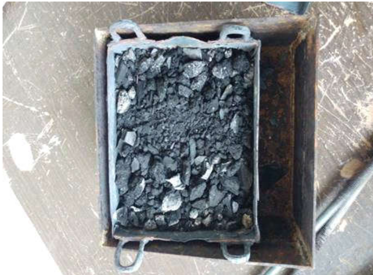
Fig. 8. Closed container (seen here with the lid open) to prevent oxidation of charcoal
