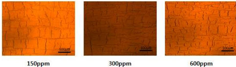
Fig. 9. Hydrogen contents-dependent microstructure variation.
