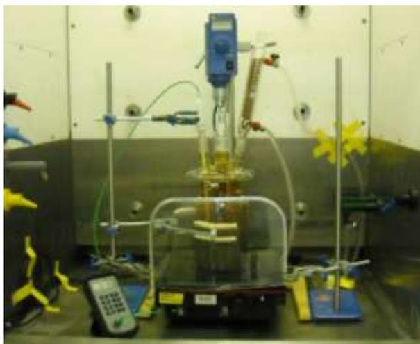
Fig 3. The “standard” Phase 2 leach apparatus.
