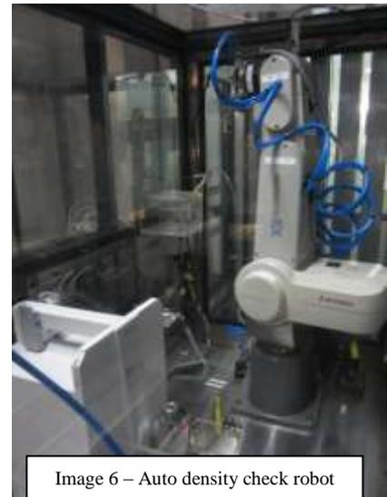
instructed to proceed by the central control system. Manual intervention is required should an unsatisfactory density result be recorded.
