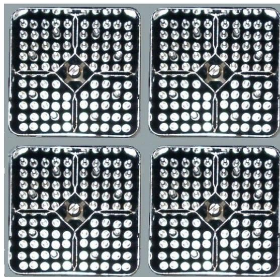
**Figure 2:** BWR fuel assembly cell. Each cell consist on four adjacent elements with a cruciform control rod in the centre.
