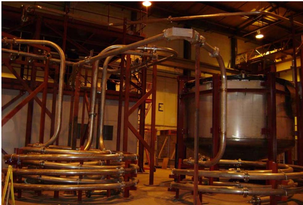
Figure 6. Full scale inactive mock-up rigs of HA Evaporator C steam heating coil and vessel base at NNL Laboratory, UK.
