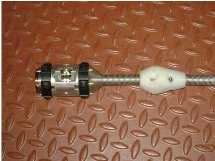
Figure 10. HA evaporator C base inspection vehicle tool package
