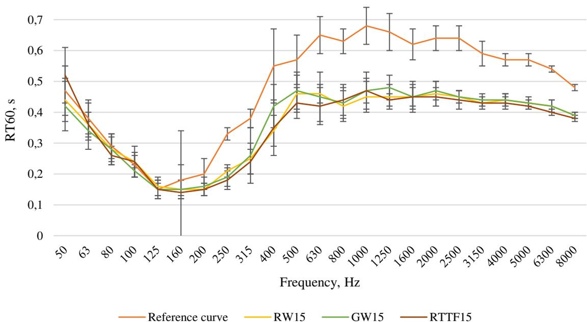
Fig. 3.8 Reverberation time reduction of 15 cm thickness by different materials
