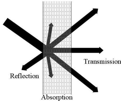
Fig. 1.5 Schematic view of sound absorption in porous materials (Bujoreanu et al., 2017)
