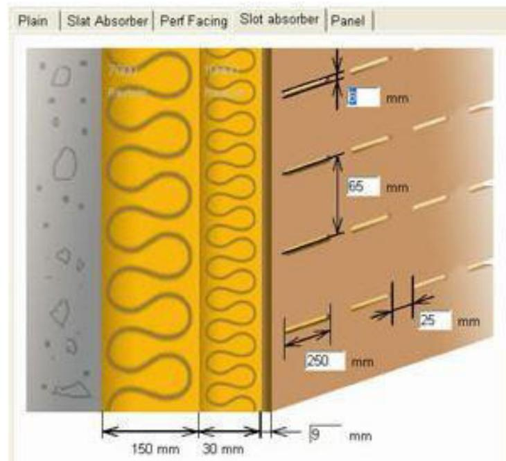
Fig. 1.20 Input data which can be inserted for calculations (screenshot from software) (Zorba, 2019b)
