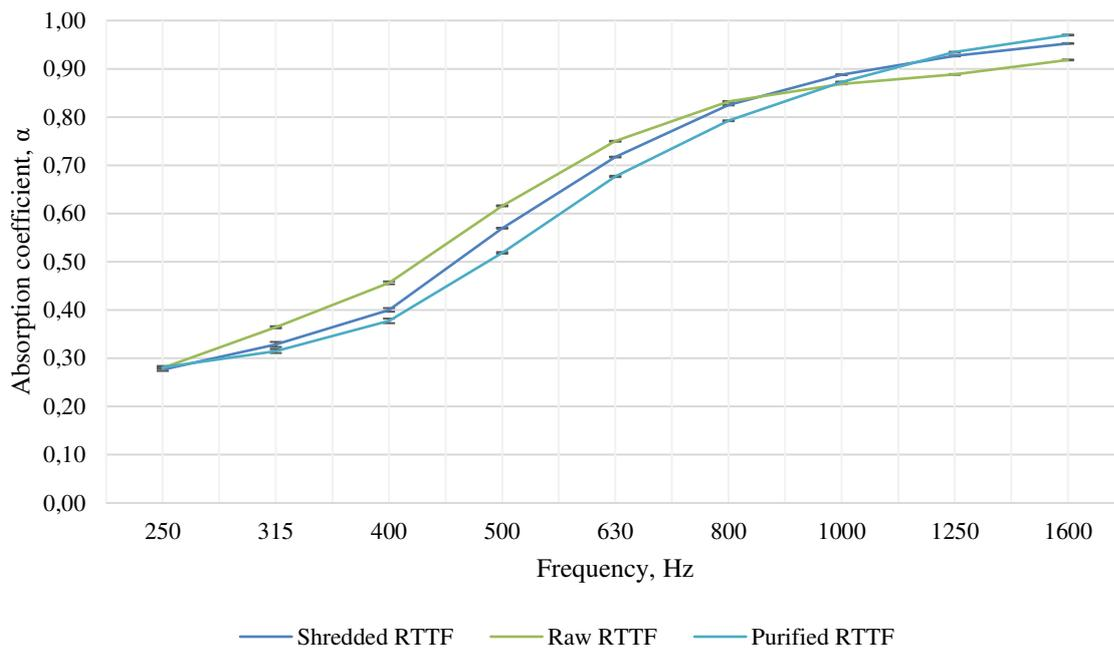
Fig. 3.16 Comparison of non-conventional materials options: shredded RTTF vs. raw RTTF vs. purified RTTF (Created by the author, 2020)
