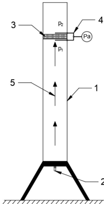
Fig. 4.1 Test stand for air flow resistivity principle scheme: 1 – air flow resistivity tube shell, 2 – inlet for air compressor, 3 – sample in the sample holder, 4 – differential pressure gauge, 5 – air flow movement direction (Created by the author, 2020)
