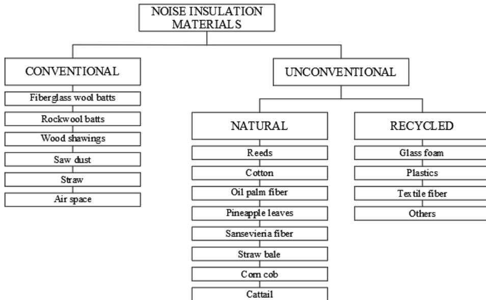
Fig. 1.3 Noise insulation materials classification (Created by the author, 2019; Asdrubali, D’Alessandro and Schiavoni, 2015)
