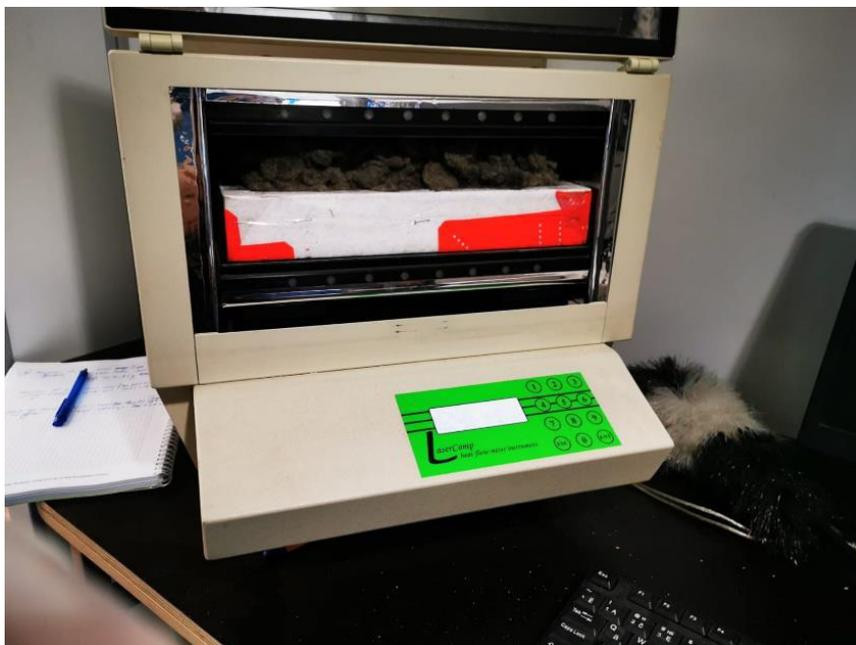
Fig. 2.8 LaserComp Heat flow meter instrument (Created by the author, 2020)
