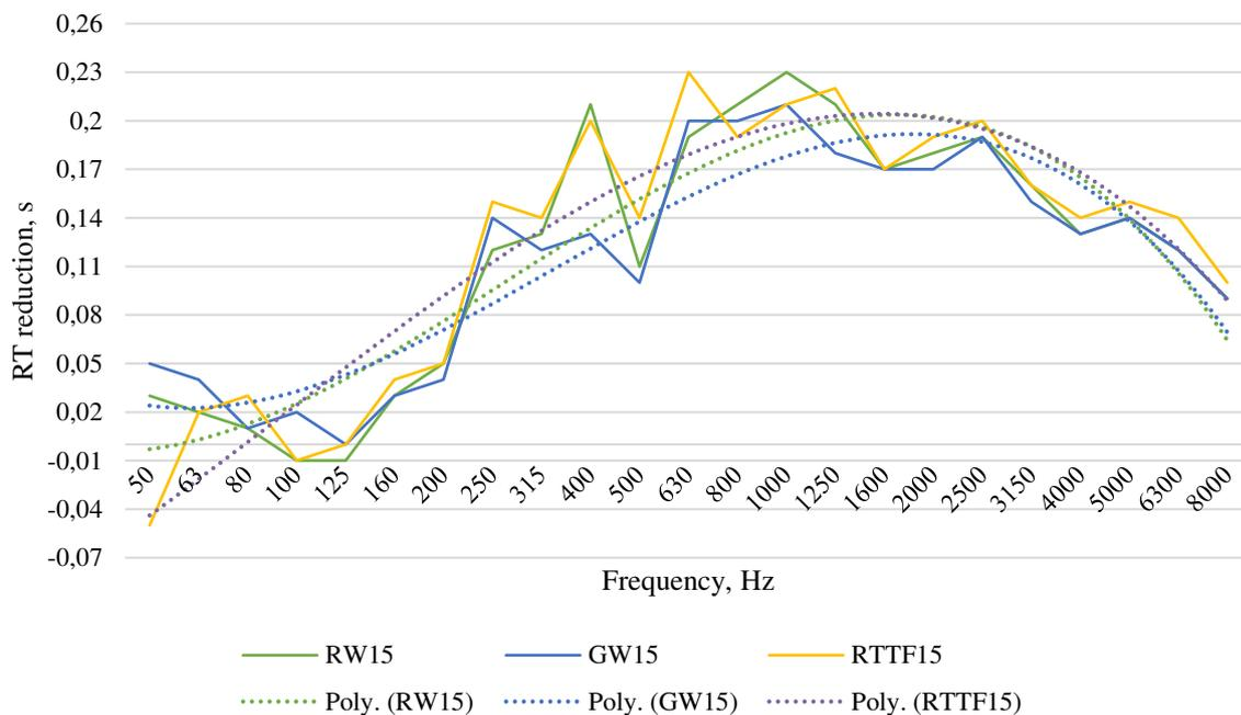
Fig. 3.9 Reverberation time reduction regarding materials 15 cm thickness
