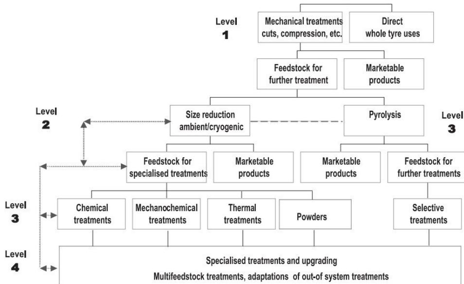
Fig. 1.18 The principal scheme of tyre recycling (Shulman, 2011)
