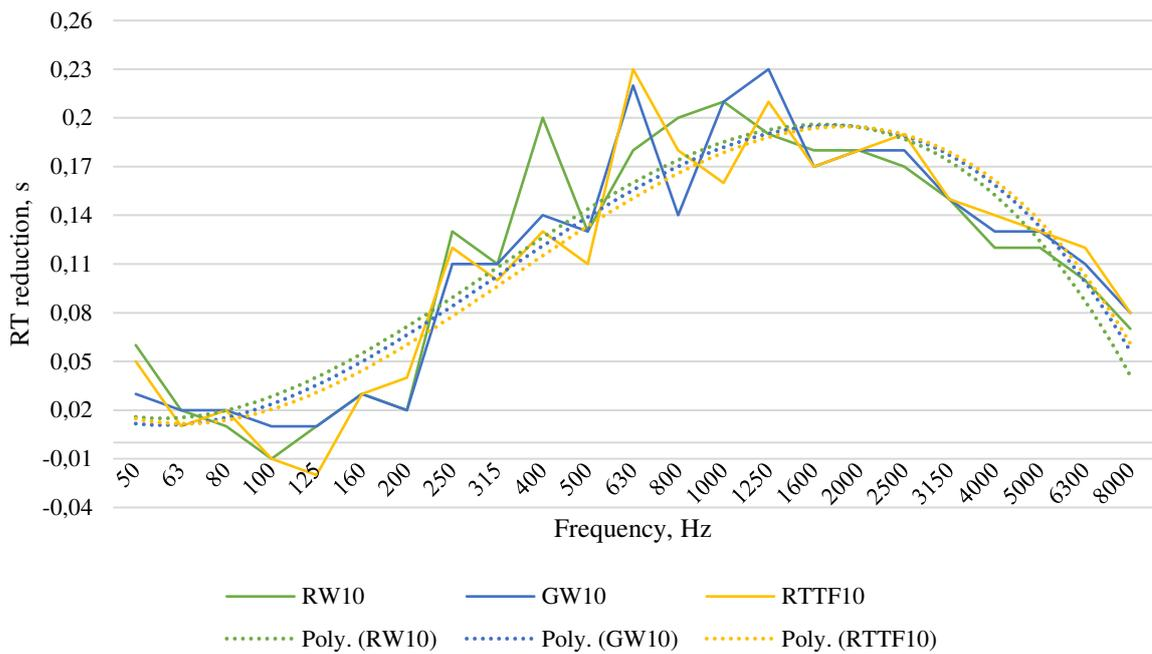
Fig. 3.7 Reverberation time reduction regarding materials 10 cm thickness
