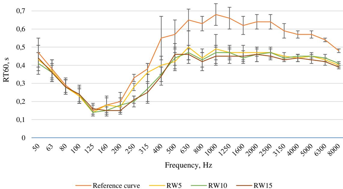
Fig. 3.1 Reverberation time difference on RW thickness (Created by the author, 2020)
