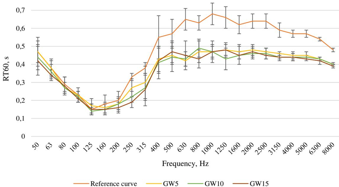
Fig. 3.2 Reverberation time difference on GW thickness (Created by the author, 2020)
