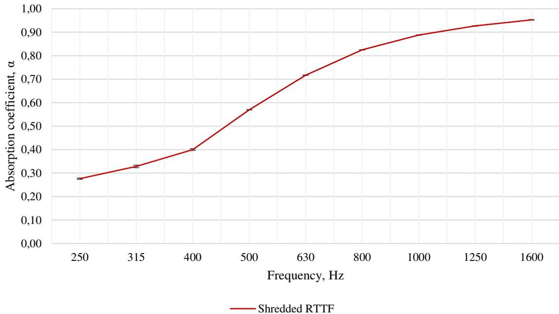
Fig. 3.13 Shredded recycled tyre textile fibre sound absorption results
