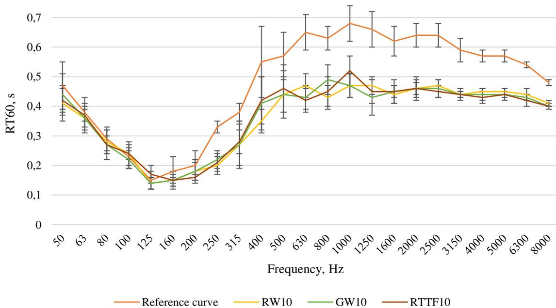
Fig. 3.6 Reverberation time reduction of 10 cm thickness by different materials
