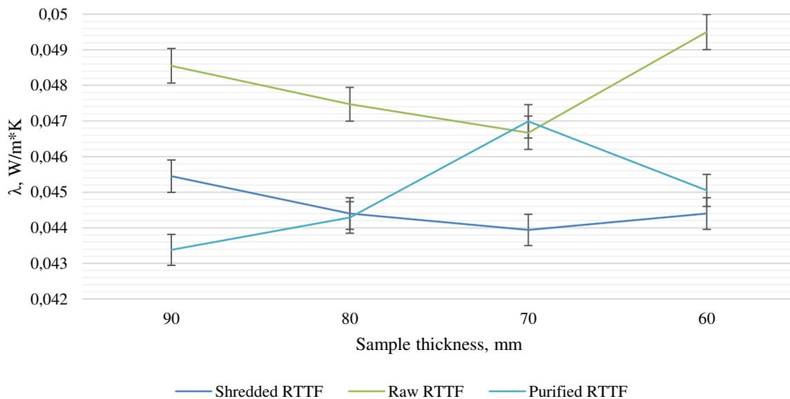
Fig. 3.21 Thermal conductivity comparison of different RTTF forms (Created by the author, 2020)
