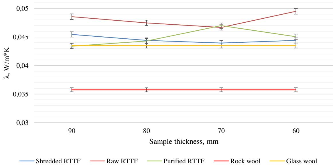
Fig. 3.22 Thermal conductivity comparison to conventional materials
