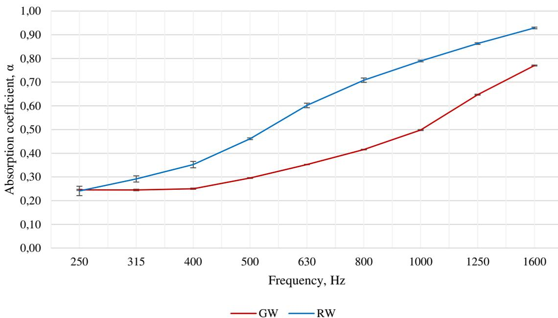
Fig. 3.12 Comparison of two conventional materials: rock wool vs. glass wool (Created by the author, 2020)
