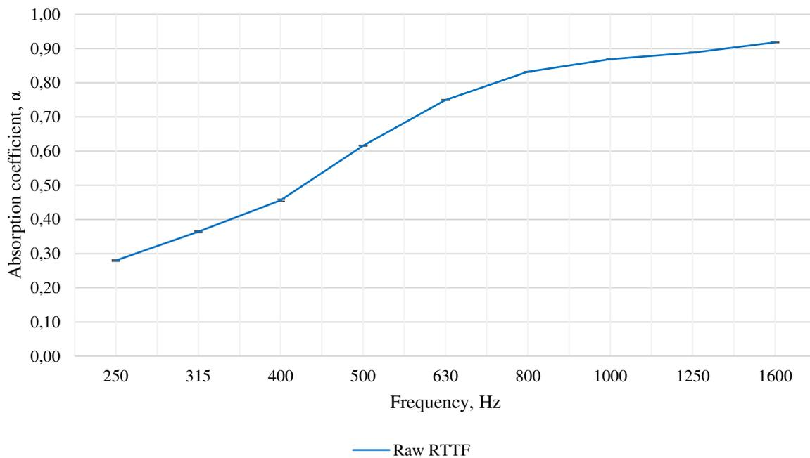
Fig. 3.14 Raw recycled tyre textile fibre sound absorption results (Created by the author, 2020)
