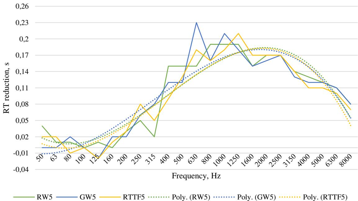
Fig. 3.5 Reverberation time reduction regarding materials 5 cm thickness
