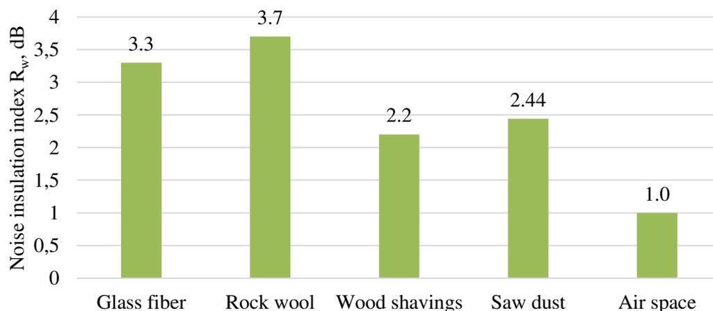
Fig. 1.4 Acoustical properties of materials at thickness of 2,54 cm (Asdrubali, D’Alessandro and Schiavoni, 2015)
