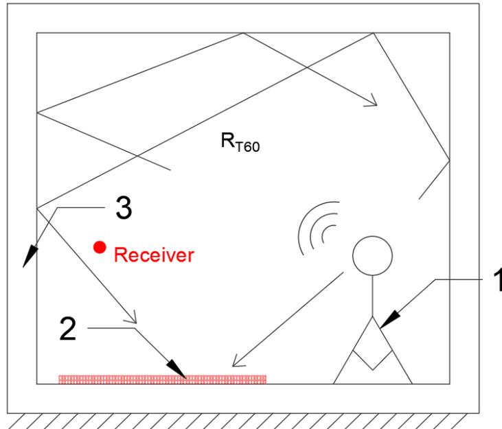
Fig. 2.3 Principle scheme of reverberation time measurements: 1 – airborne noise source; 2 – sound absorbing sample; 3 – reverberation room,  $R_{T60}$  – reverberation time, s
