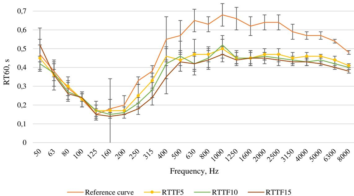
Fig. 3.3 Reverberation time difference on RTTF thickness (Created by the author, 2020)
