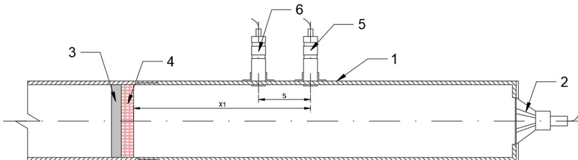
Fig. 2.4 Impedance tube principle scheme: 1 – impedance tube shell (acrylic glass), 2 – sound speaker, 3 – rigid backing, 4 – sound absorption sample, 5 – microphone No. 1, 6 – microphone No. 2 (Created by the author, 2020)
