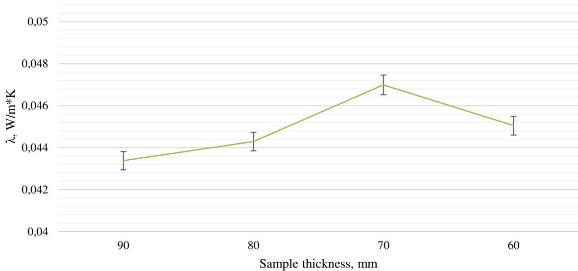
Fig. 3.20 Thermal conductivity change on the compression ratio of purified RTTF
