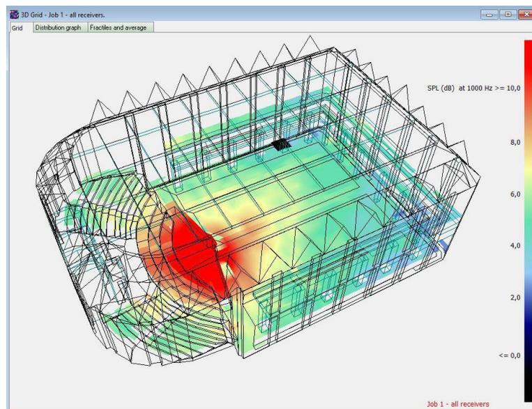
Fig. 1.19 ODEON results of SPL results (screenshot from software) (ODEON, 2019)
