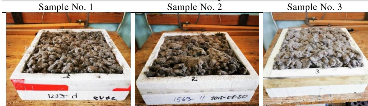
Thermal conductivity of the sample is determined in the heat flow meter equipment. Thermal conductivity is determined by the measuring of the heat flux, sample thickness, and temperature difference through the sample. Thermal conductivity measured by the heat flux transducers, which are placed on heating or cooling plates. The thickness measurement precision is 0.002 cm, and temperature 0.01 °C. Principle scheme of the measurement presented in Fig. 2.6.
