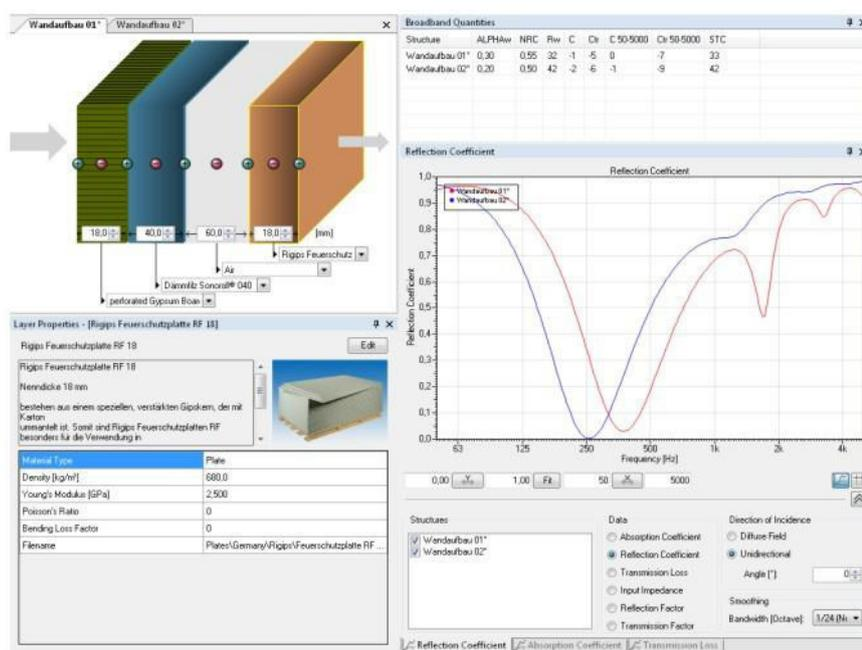
Fig. 1.21 AFMG SoundFlow software main window (screenshot from software) (AFMG SoundFlow, 2019)
