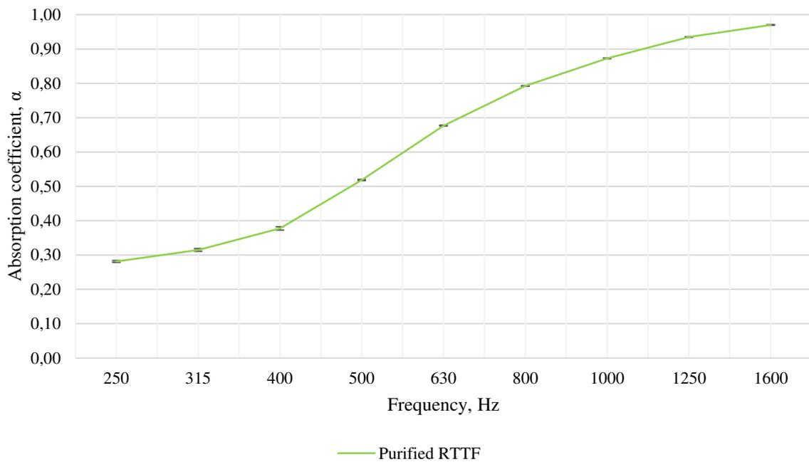
Fig. 3.15 Purified recycled tyre textile fibre sound absorption results
