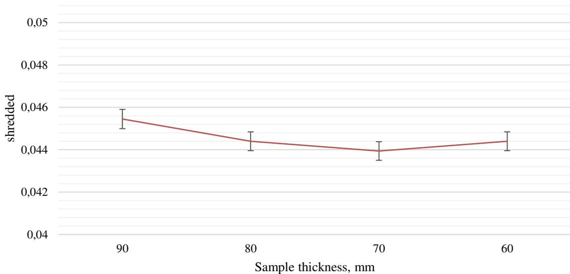
Fig. 3.18 Thermal conductivity change on the compression ratio of shredded RTTF
