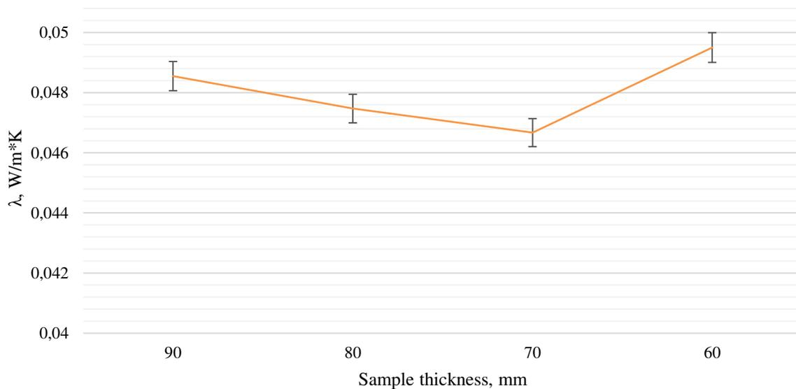
Fig. 3.19 Thermal conductivity change on the compression ratio of raw RTTF (Created by the author, 2020)
