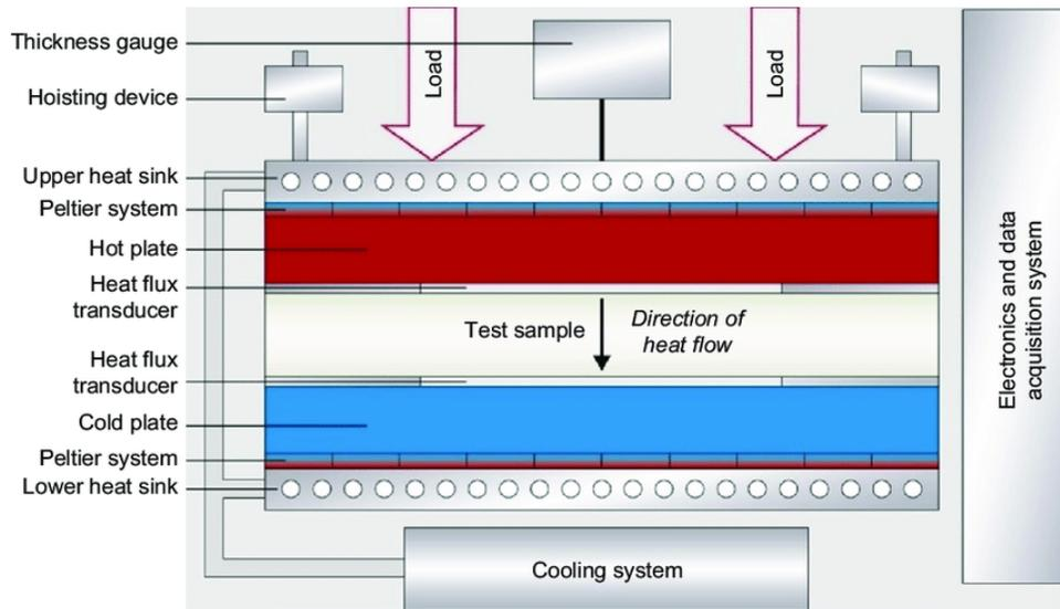
Fig. 2.5 Thermal conductivity meter principle scheme (Ugovšek and Šubic, 2017)
