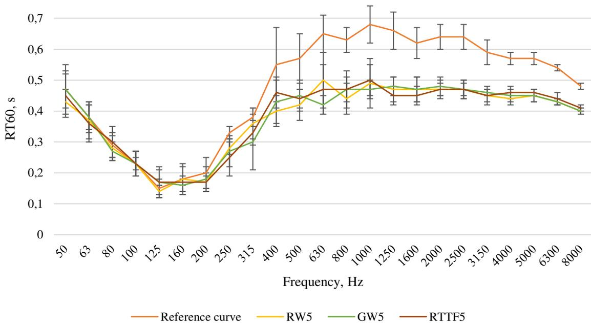
Fig. 3.4 Reverberation time reduction of 5 cm thickness by different materials
