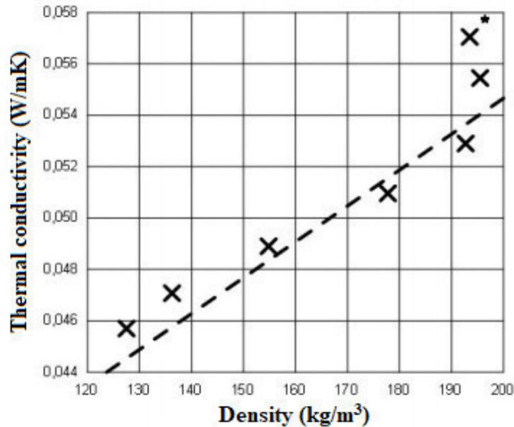
Fig. 1.6 Correlation of density and thermal conductivity (Bozsaky, 2012)
