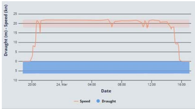
Figure 2. Ro-Pax ship's “Victoria Seaways” speed distribution during the voyage Klaipeda – Kiel” (AIS information)
