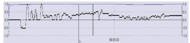
Fig. 13. Hydrodynamic influence between the PANAMAX tanker and a ferry expressed as rudder rotation in the narrow channel in the parallel direction (vertical line in the figure corresponds to the ship position in Fig. 12)
