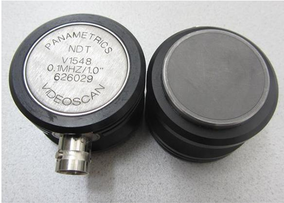
**Figure 7.2:** Longitudinal Transducers
