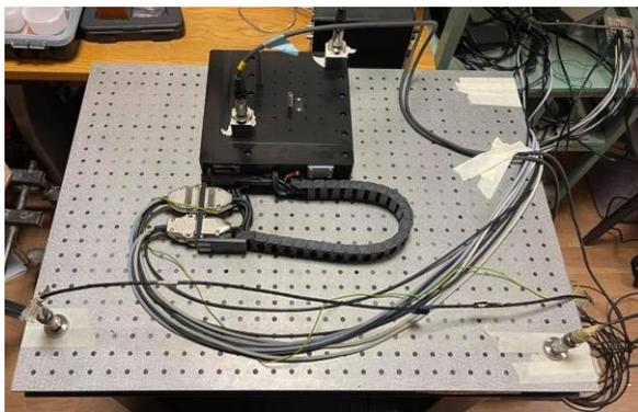
**Figure 6** Experimental setup of precision positioning system with linear motor dynamic processes
